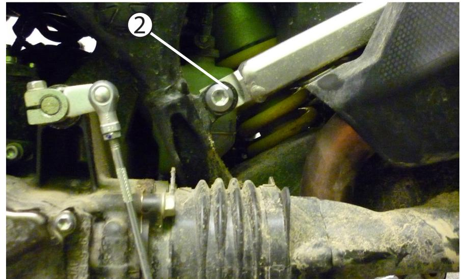
② Using a 14mm wrench and t50 torx tool, remove the nut on the back of this fastener. Leave the OEM fastener in place, just pull the nut off of the back.
