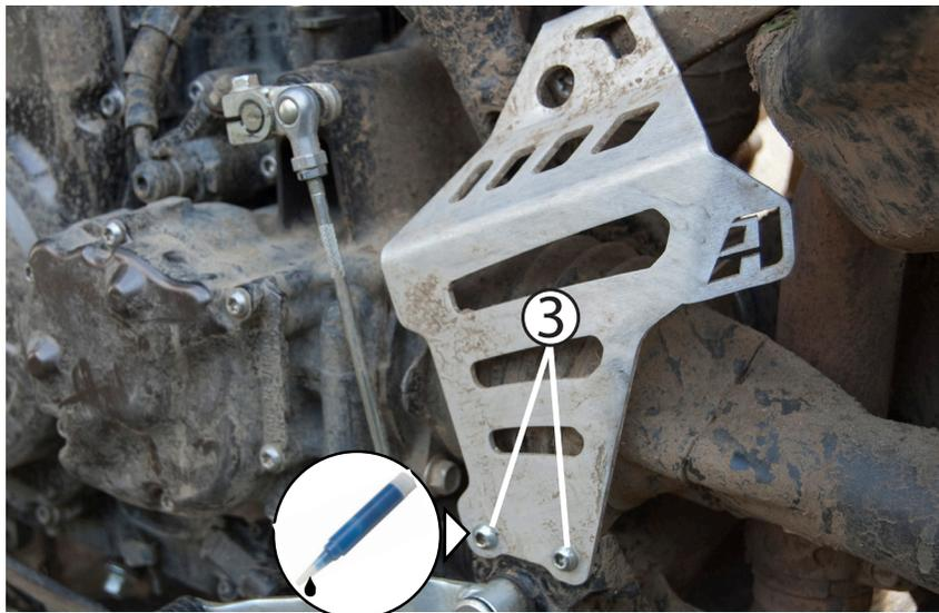
③ Install the AltRider Universal Joint Guard. After applying thread locker to the last couple of threads on the (2) OEM fasteners, use a 4mm allen tool to tighten these down. Make sure the tab on the top is lined up with the OEM bolt.
