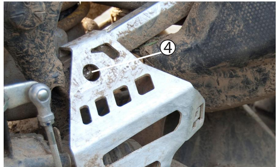
④ After applying a drop of thread locker to the inside of the OEM nut, use the 14mm wrench and t50 torx tool to tighten it down.
